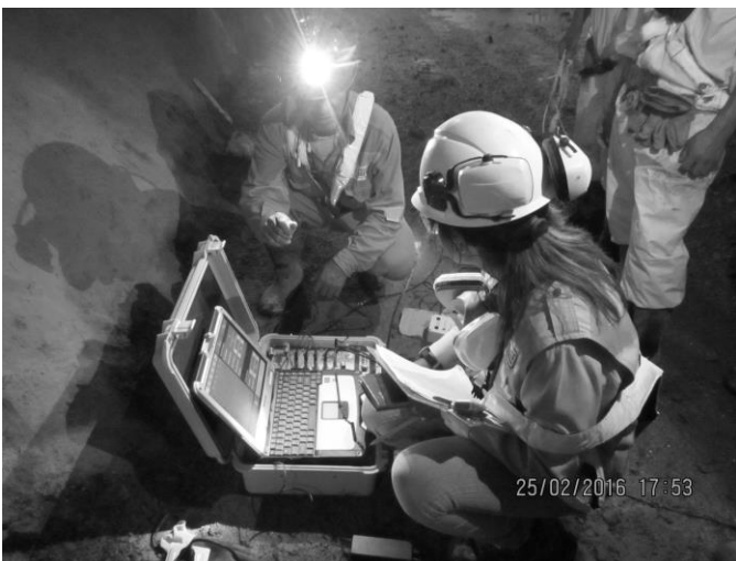
Figure 28: DNA -BLAST engineer recording on the tunnel by TSP method.
