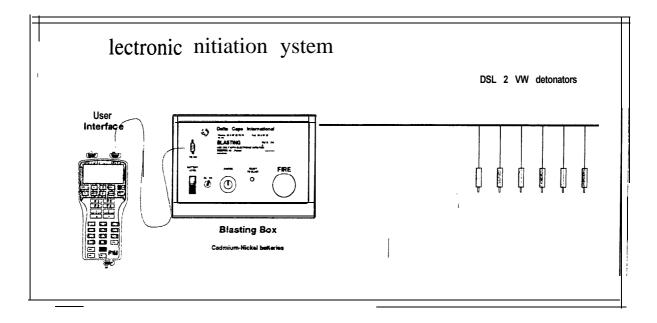
DSL2 EID (Electronic Initiation Devices) are controlled by the blasting box.
